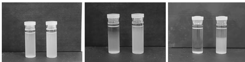
Fig. 9. Comparison of colloidal stabilities of bare MDH particles (left vial) and MDH-poly( n butyl acrylate) particles in THF (Initial, after 2 h and 2 weeks; from left).
